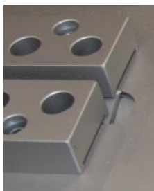
Figure 4: Notches between the pressure strip and back
